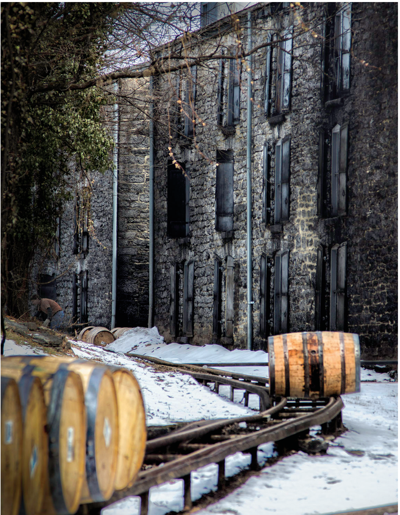
Barrels on a run, Old Oscar Pepper Distillery/Labrot and Graham Distillery, Woodford County. The historical warehouses of Old Oscar Pepper Distillery are the backdrop for the well-known 1934 Labrot and Graham elevated barrel runs, constructed after Prohibition and continued to be used today. They are famous for being completely gravity-driven.
